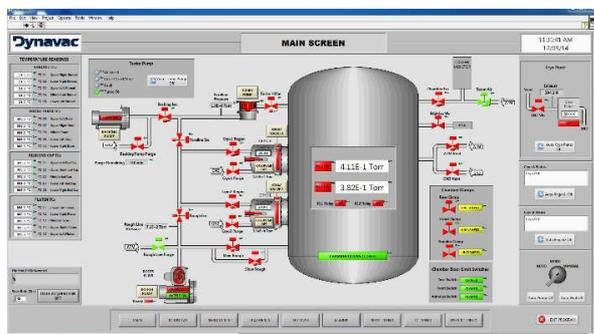
Figure 8: S2F Control HMI - System Status & Control
