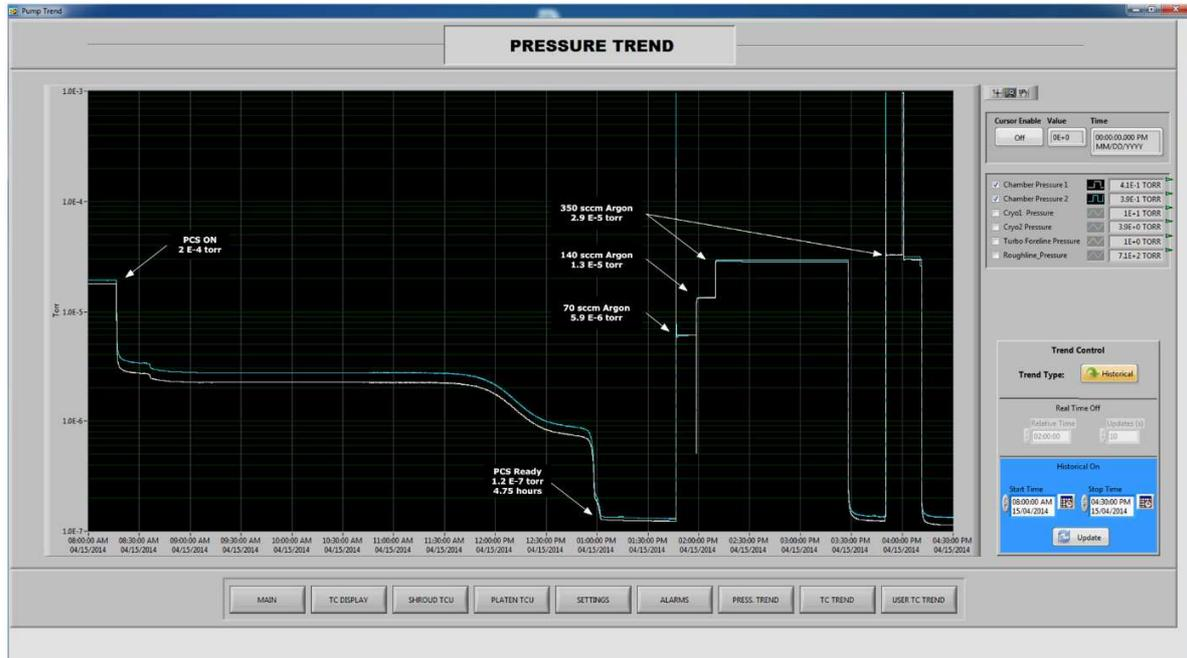
Figure 17: PCS Acceptance Test Results – Argon Fuel
