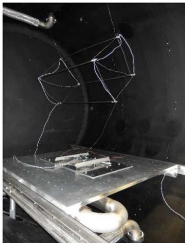
*Figure 10: Thermal Platen with Test Heaters*
