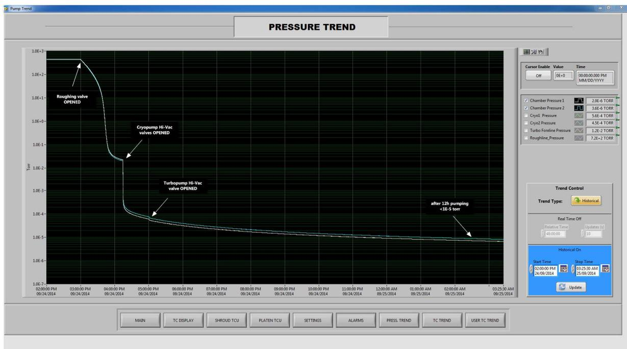
Figure 15: S2F Typical Chamber Pumpdown Plot (“wet chamber”)
