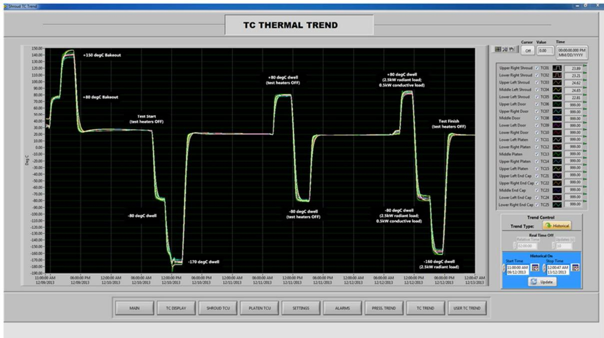
Figure 16: S2F TVAC Acceptance Test Results
