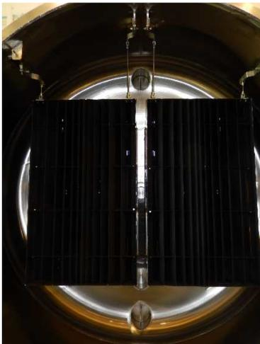
*Figure 13: PCS Pumps Mounted to Rear Endcap*
