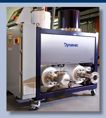
Dynavac Gaseous Nitrogen Thermal Conditioning Units are operating in aerospace facilities around the globe providing exacting control of thermal vacuum test environments.
