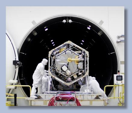
Dynavac manufactures thermal vacuum systems that simulate the harsh conditions of space. Our systems are designed to replicate a variety of environmental conditions and performance criteria for prequalification of space flight hardware.
