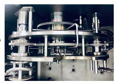
The resulting water-cooled mechanism supports single or planetary configurations. A substrate or a tooling plate is mounted directly to a water-cooled jacket and is held at the specified substrate temperature during deposition. A supervisory control system fully automates the closed-loop cooling water and independent chiller. Input and output water temperature is captured and logged. The USPTO has granted a provisional patent for the innovative aspects of the mechanism.
